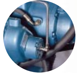
Thrust balance pistons on low and high pressure compression elements equalise bearing loads and extend element life
